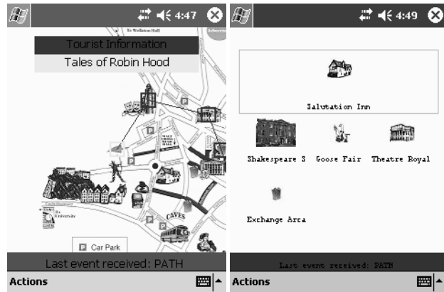
Figure 3: Feedback styles presented on the PDA during interaction with the Nottingham map. On the left is the map-style feedback, indicating that a path has been selected for a query constrained as “tourist information”. On the right is an example of “butterfly net” feedback, showing the list of items selected so far, and the current item the PDA is over.
