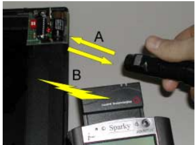
Figure 1: Line-of-sight identification with tag and gesturePen . A: The user points to a tag with a special pen to uniquely identify a laptop (e.g. its network address). B: Information can then be transferred over a wireless network to the laptop
